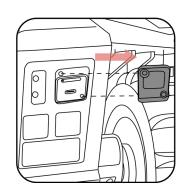
2. Eject the SIM card tray using the SIM-eject tool, install the SIM card, and push the card tray into place.
