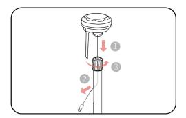
5. Secure the charging station on the flat surface using the five stakes. Place a gasket onto the inlet, then insert and fix the trident ground stake as shown in the figure and keep it upright.
