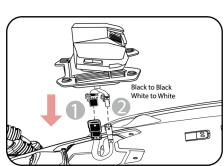
3. Attach the vision module to the Luba using the four screws and tighten them with a 2.5mm hex screwdriver.
