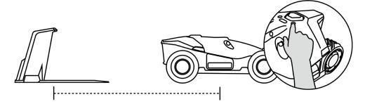
• Move Luba onto the charging station and wait for Luba to power on automatically.
